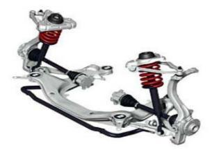
**Figure 1.3 -** Suspension de type double triangulation [5]
