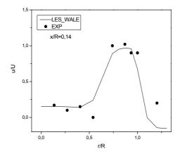
**Figure 4.6 (a).** Radial profiles of mean axial velocity and axial fluctuation intensity (x/R=0.14).
