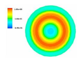
Figure 4.7(b). Iso-surface of the axial velocity (x/R=0.38).
