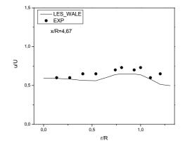
*Figure 4.6(c).* Radial profiles of mean axial velocity and axial fluctuation intensity (x/R=4.67).
