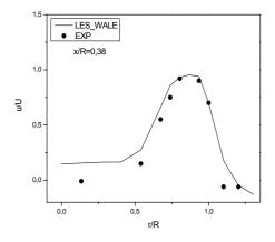
**Figure 4.6(b).** Radial profiles of mean axial velocity and axial fluctuation intensity (x/R=0.38).
