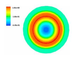
Figure 4.7(a). Iso-surface of the axial velocity (x/R=0.14).
