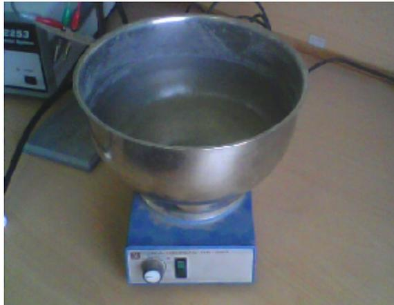
*Figure IV.11: Thermostat (model IKA-HEIZBAD HB-250, Max300C°)*
