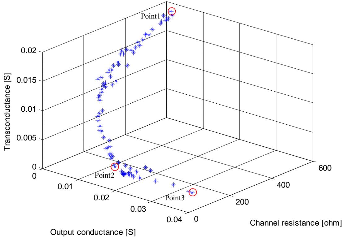
Figure V.11: Pareto-optimal solutions of the analyzed DM GaAs- MESFET
