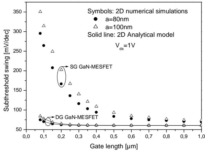
Figure IV.6: Subthreshold swing factor as function of channel length for different active region thicknesses. Device parameters used for calculating are  $\phi_M = 4.68eV$ ,  $V_{bi} = 1.1V$ ,  $N_d = 3.10^{17} cm^{-3}$ ,  $V_{ds} = 1V$ .
