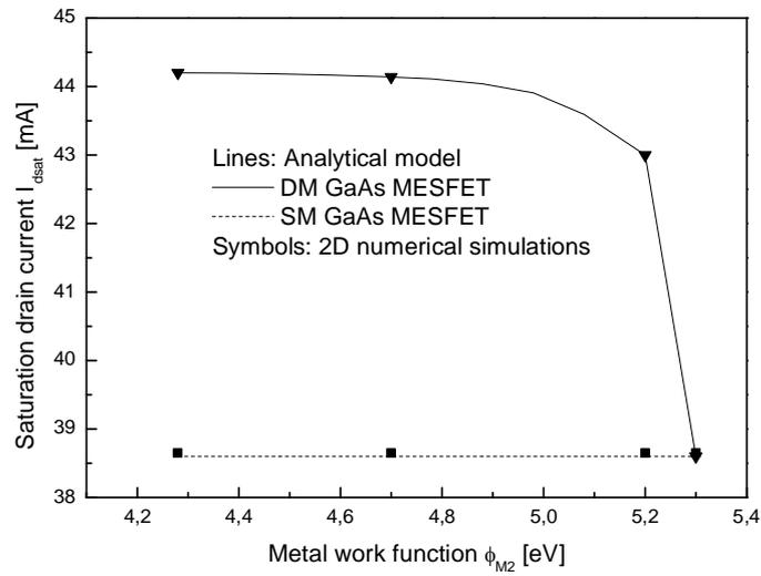
Figure V.9: variation of the saturation drain current,  $I_{dsat}$ , as function of metal gate work function near the drain end,  $\phi_{M2}$ , for a fixed  $V_{gs} = 0V$ ,  $V_{ds} = 6V$ ,  $\phi_{M1} = 5.3eV$  and  $L_1 = 0.1\mu m$ .
