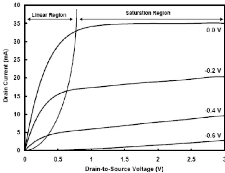
Figure II.4: Typical  $I$ - $V$  characteristics of a GaAs MESFET showing linear and saturation regions.
