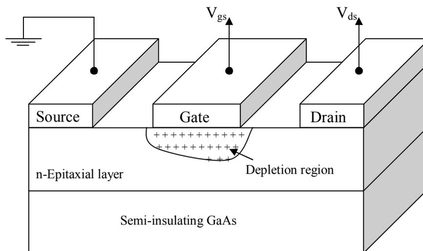
Figure II.2: A cross-sectional view of a GaAs MESFET fabricated on a semi-insulating GaAs substrate
