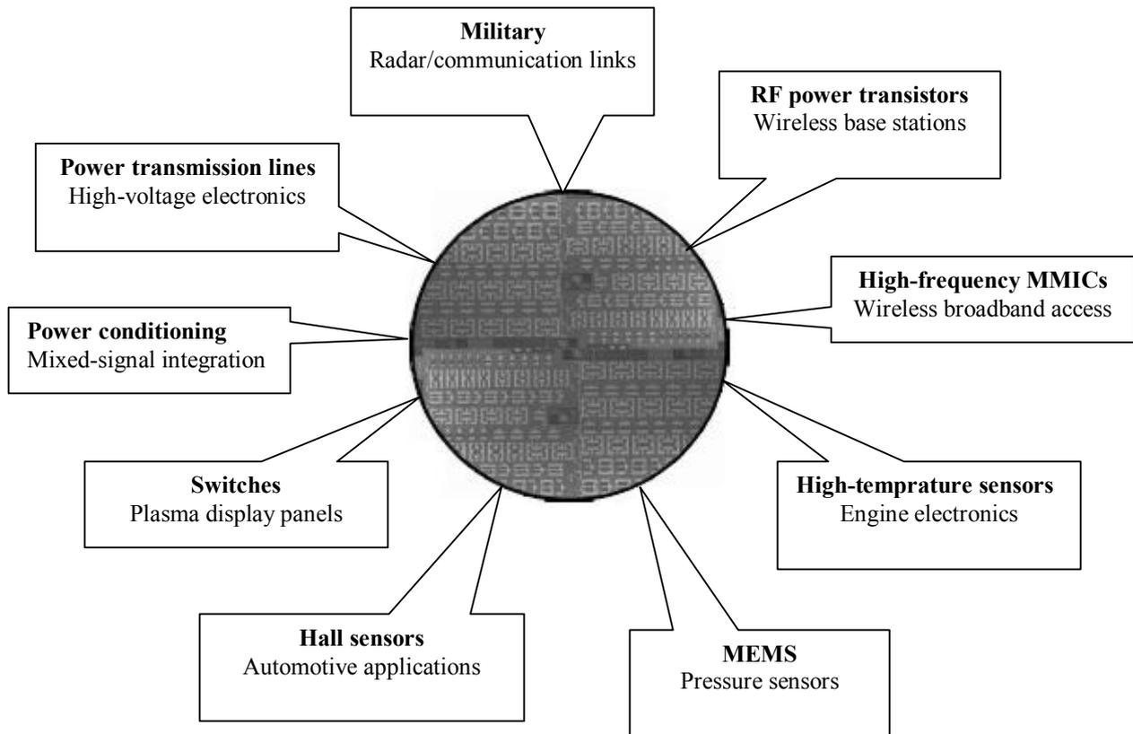
Figure I.3: GaN-based micro-electronic applications [35].
