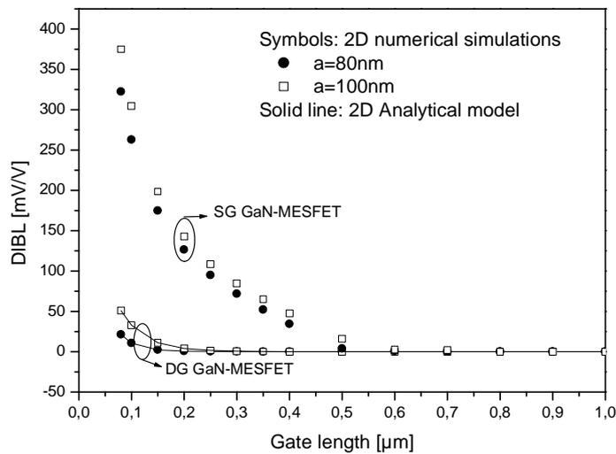
Figure IV.5: Drain induced barrier lowering, DIBL, coefficient as function of channel length for different active region thicknesses.
