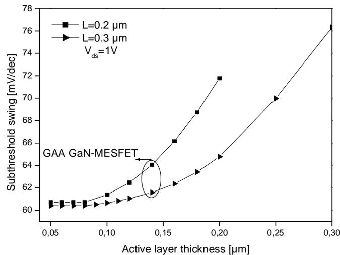
Figure IV.12: Subthreshold swing factor as function of channel thickness (diameter) for different channel lengths. Device parameters used for calculating are  $\phi_M = 4.68\text{eV}$ ,  $V_{bi} = 1.1\text{V}$ ,  $N_d = 3.10^{17}\text{ cm}^{-3}$ ,  $V_{ds} = 1\text{V}$ .
