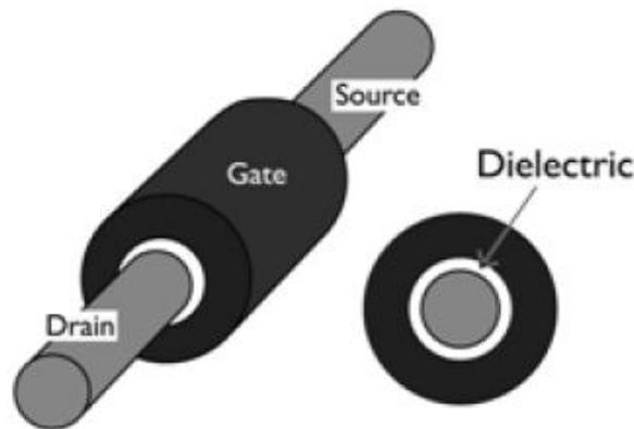
*Figure II.8: Gate-All-Around FET structure*
