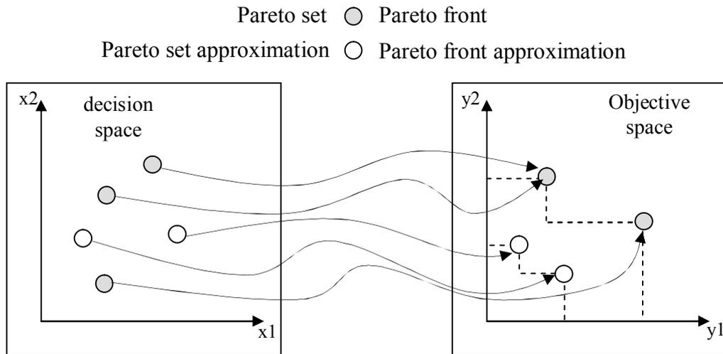
Figure III.5: Mapping from decision space to objective space - assuming maximization
