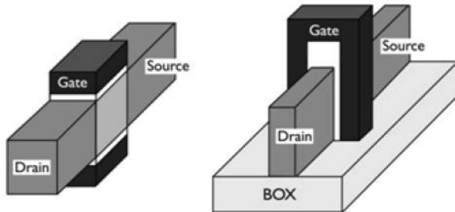
Figure II.6: Dual-Gate FET structure (left) and a FinFET structure (right)
