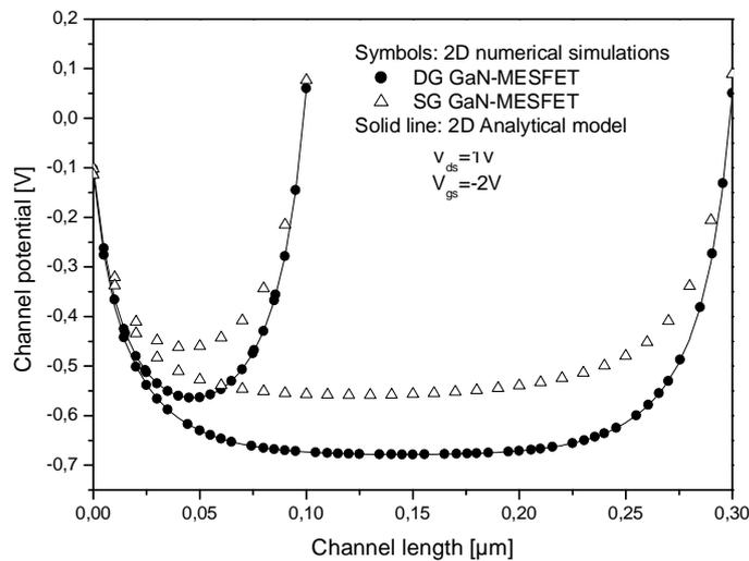
Figure IV.3: Potential variation along the channel of the (DG) GaN-MESFET and conventional GaN-MESFET for different channel lengths. Device parameters used for calculating are  $V_{ds} = 1V$ ,
