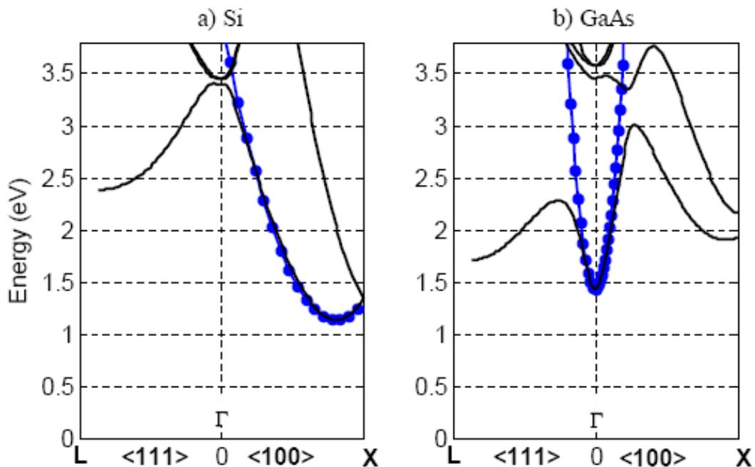
Figure I.1: Electronic band structure of two common semiconductors calculated for the bulk case [21], and their respective parabolic fit (circles). Zero energy corresponds to the top of the valence band. a) Si conduction band is shown with a parabolic fit in the X direction corresponding to  $m^*=0.91m_0$ . b) GaAs band structure showing the parabola at the point where the effective mass is very light ( $m^*=0.067m_0$ ).
