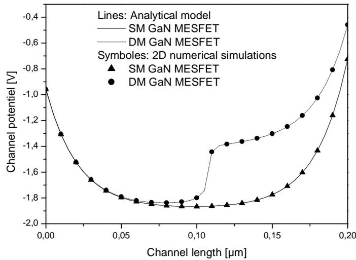
Figure V.2: Potential variation along the channel of the DM GaN-MESFET and conventional SM GaN-MESFET. Device parameters used for calculating are  $V_{ds} = 1V$ ,  $V_{gs} = -1V$ ,  $a = 100nm$ ,  $\phi_{M1} = 5.1eV$ ,  $\phi_{M2} = 4.68eV$ ,  $V_{bi1} = 1.6V$ ,  $V_{bi2} = 1.1V$ ,  $N_d = 3.10^{17} cm^{-3}$
