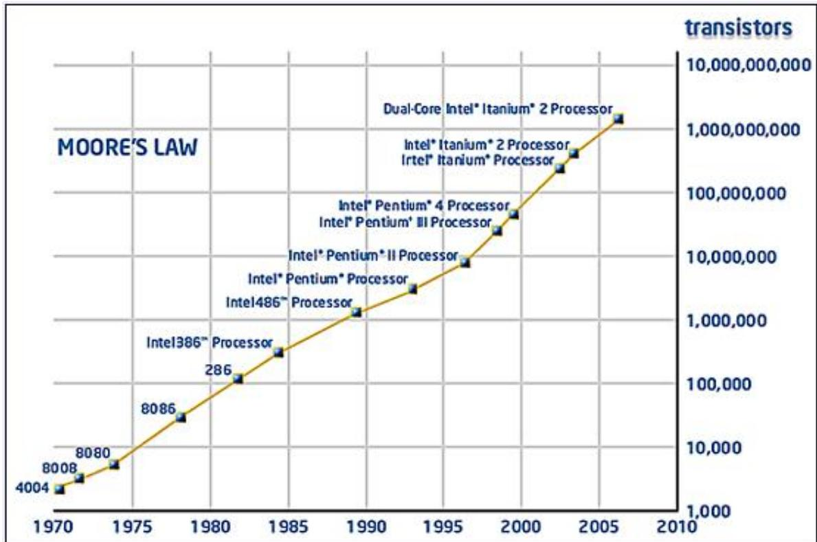
Figure II.1: Increasing number transistors with each new microprocessor technology [42]
