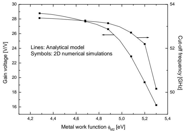
Figure V.12: variation of voltage gain and cut-off frequency as function of metal gate work function near the drain end,  $\phi_{M2}$ , for a fixed  $\phi_{M1} = 5.3\text{eV}$  and  $L_1 = 0.1\mu\text{m}$ .
