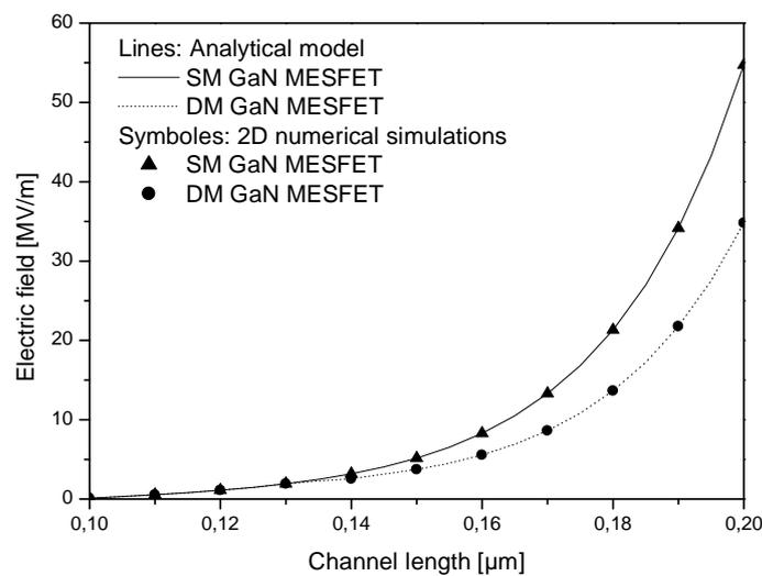
Figure V.3: Electric-field variation along the channel of DM and SM GaN-MESFETs for a channel length  $L=0.2\mu m$  ( $L_1 = L_2 = 0.1\mu m$ ).
