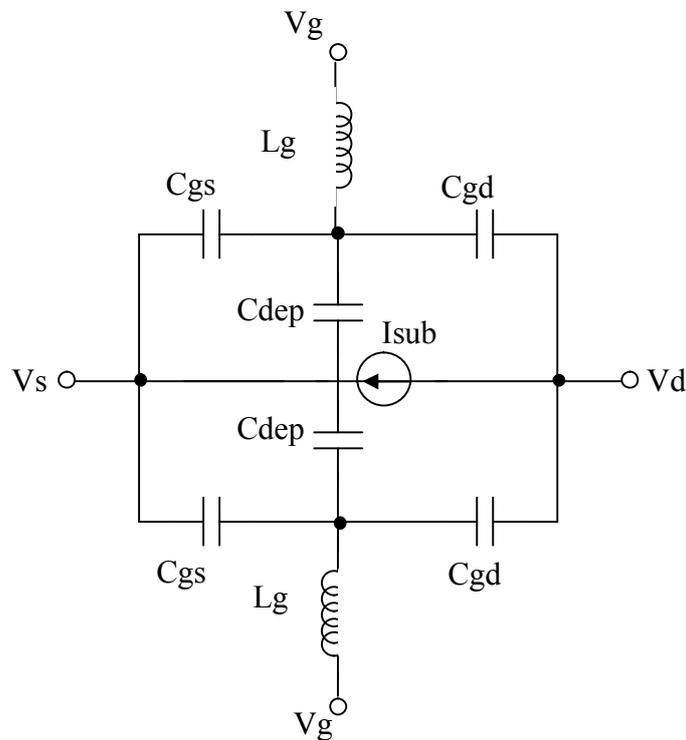
Figure IV.7: Electric scheme of the DG GaN-MESFET without parasitic resistances
