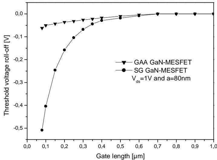
Figure IV.9: Threshold voltage roll-off versus channel length of GAA GaN-MESFET and conventional planar GaN-MESFET. Device parameters used for calculating are  $a = 80nm$ ,  $\phi_M = 4.68eV$ ,  $V_{bi} = 1.1V$ ,  $N_d = 3.10^{17} cm^{-3}$ ,  $V_{ds} = 1V$ .
