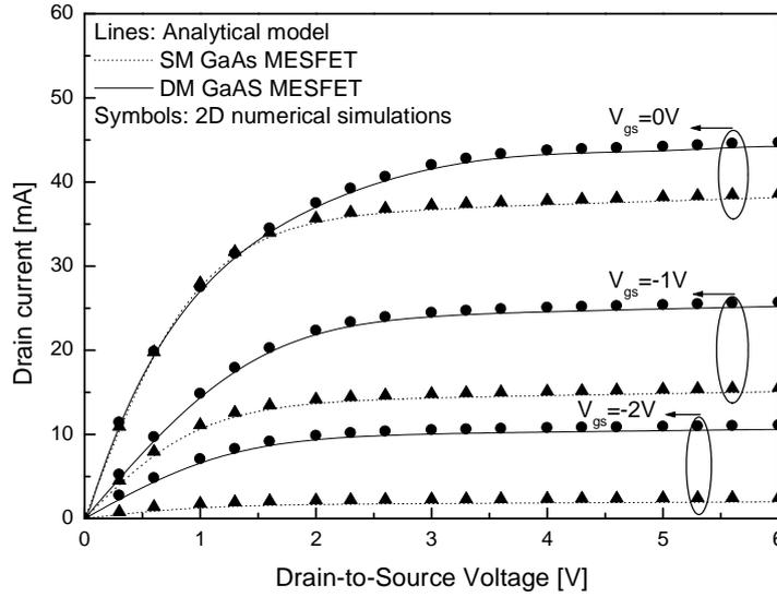
Figure V.8: Output characteristics for a channel length of a  $0.2 \times 200 \mu\text{m}^2$  ( $L_1 = 0.1 \mu\text{m}$ ) DG GaAs-MESFET compared with that of the conventional SM GaAs-MESFET. Device parameters used for calculating are  $a = 0.1 \mu\text{m}$ ,  $\phi_{M1} = 5.3 \text{eV}$ ,  $\phi_{M2} = 4.28 \text{eV}$ ,  $V_{bi1} = 1.3 \text{V}$ ,  $V_{bi2} = 0.21 \text{V}$ ,  $N_d = 5.10^{17} \text{cm}^{-3}$ .
