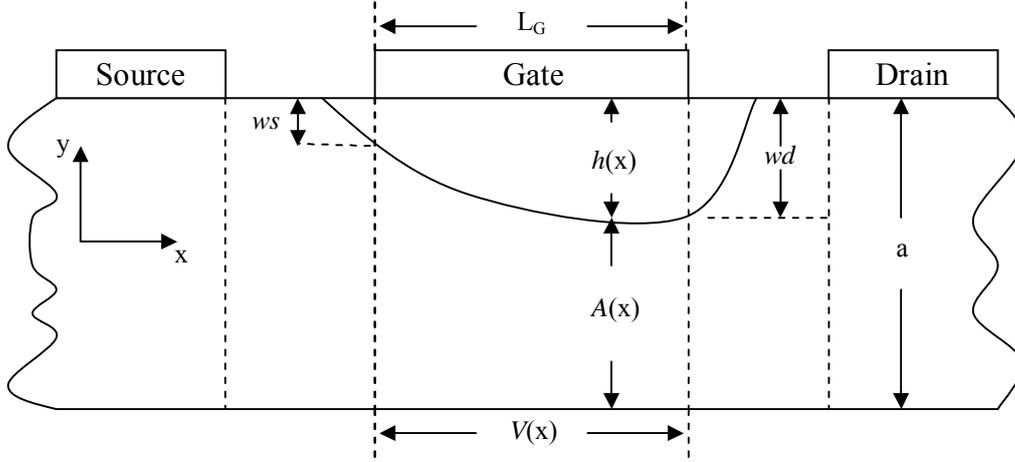
Figure II.3: A cross-sectional view of a biased GaAs MESFET channel.
