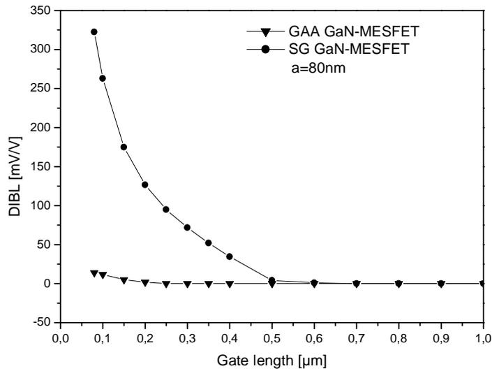
Figure IV.10: Drain induced barrier lowering, DIBL, coefficient as function of channel length for both designs (GAA and planar structure)
