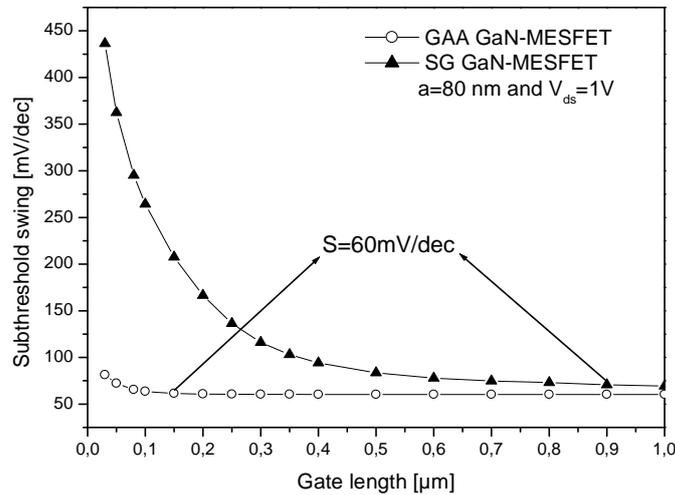
Figure IV.11: Subthreshold swing factor as function of channel length for both architectures. Device parameters used for calculating are  $\phi_M = 4.68\text{eV}$ ,  $V_{bi} = 1.1\text{V}$ ,  $N_d = 3.10^{17}\text{ cm}^{-3}$ ,  $V_{ds} = 1\text{V}$
