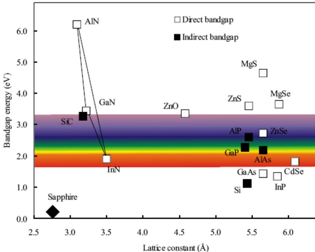
Figure I.2: Bandgap energy versus lattice constant for various semiconductors including the wide-bandgap materials SiC and GaN with its alloys [31].
