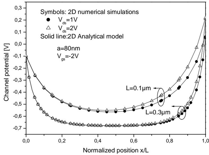
Figure IV.4: Channel potential versus normalized channel position for different drain biases and channel lengths. Device parameters used for calculating are
