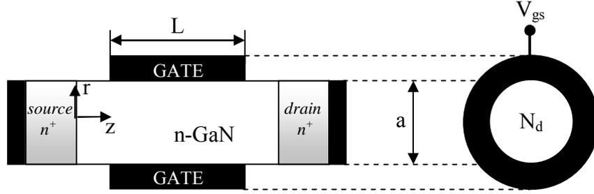
Figure IV.8: Cross-sectional view through the channel of the proposed GAA GaN-MESFET
