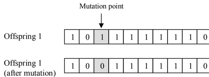
*Figure III.4: Mutation Operator*
