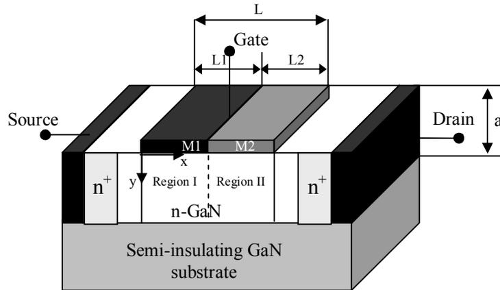
Figure V.1: Cross-sectional view of the proposed DM GaN-MESFET
