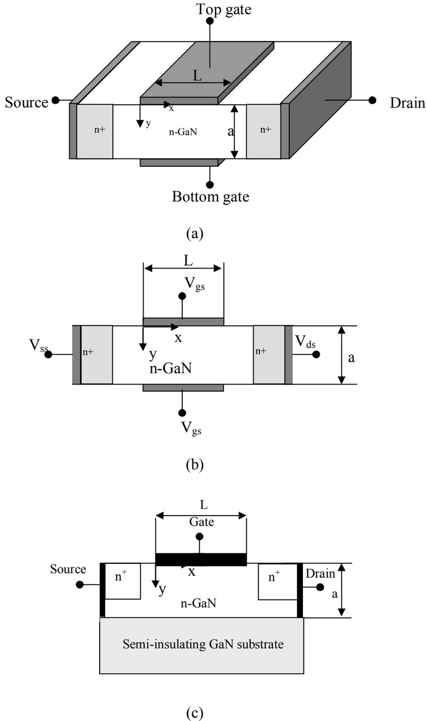
Figure IV.1: GaN-MESFET: (a) DG 3-D structure, (b) DG cross-sectional view through the channel c) SG cross-sectional view through the channel.
