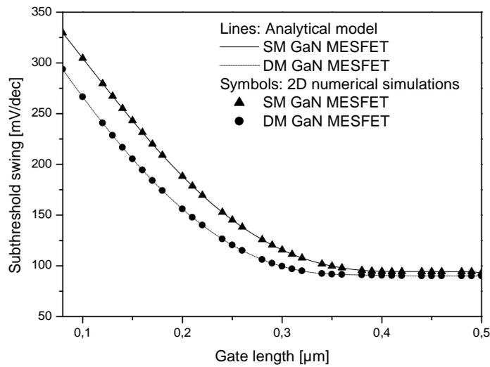
Figure V.5: Subthreshold swing factor as function of channel length for both designs. Device parameters used for calculating are
