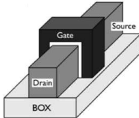
*Figure II.7: Tri-Gate FET structure [84]*
