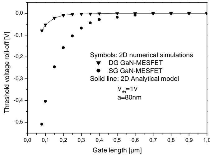
Figure IV.2: Threshold voltage roll-off versus channel length of (DG) GaN-MESFET and conventional GaN-MESFET. Device parameters used for calculating are  $V_{gs} = -2V$ ,  $a = 80nm$ ,  $\phi_M = 4.68eV$ ,  $V_{bi} = 1.1V$ ,  $N_d = 3.10^{17} cm^{-3}$ ,  $V_{ds} = 1V$ .
