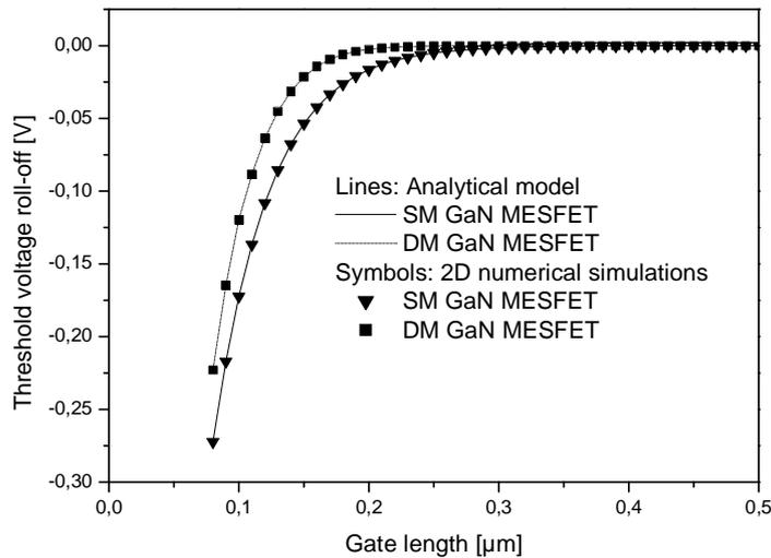
Figure V.4: Threshold voltage roll-off versus channel length of DM GaN-MESFET and conventional SM GaN-MESFET. Device parameters used for calculating are
