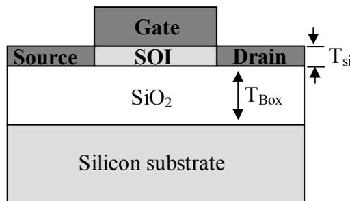
Figure II.5: Schematic diagram for UTB MOSFET [82]
