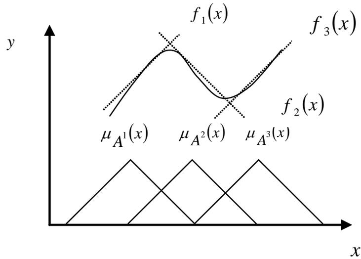
Figure 2.2: A function  $f$  defined by a T-S model
