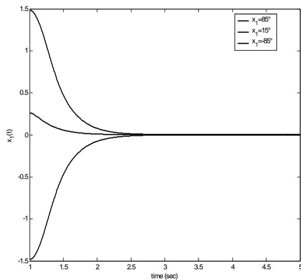
Figure 3.3: Angle response using two-rule fuzzy control for  $x_1 = 85^\circ$ ,  $15^\circ$ ,  $-85^\circ$  and  $x_2 = 0$ .
