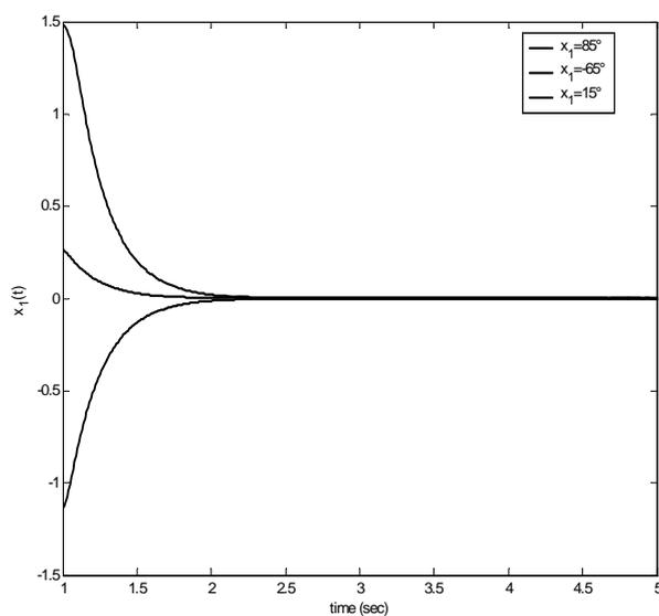
Figure 3.6: Angle response using two-rule fuzzy control and  $2l$  changed from 1.0 to 0.5  $m$ .
