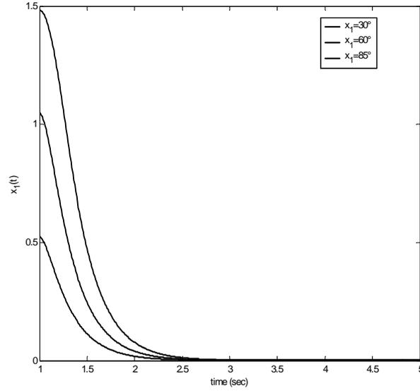
Figure 3.2: Angle response using two-rule fuzzy control for  $x_1 = 30^\circ, 60^\circ, 85^\circ$  and  $x_2 = 0$ .
