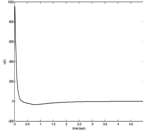
Figure 5.2: Inverted pendulum action evolution with a pole placement
