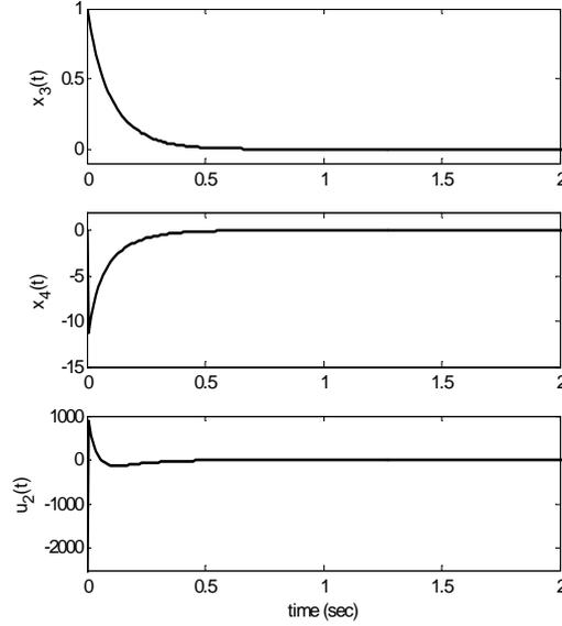
Figure 4.5: Example 4 (Two-link robot) performances: Link 2 (non-quadratic approach)
