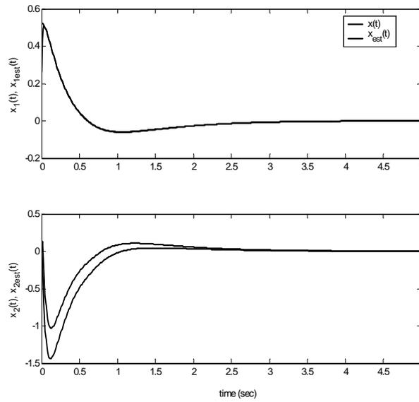
Figure 5.1: Inverted pendulum performances with a pole placement
