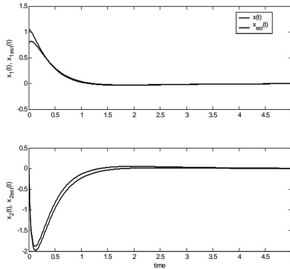
Figure 5.3: Inverted pendulum performances without pole placement
