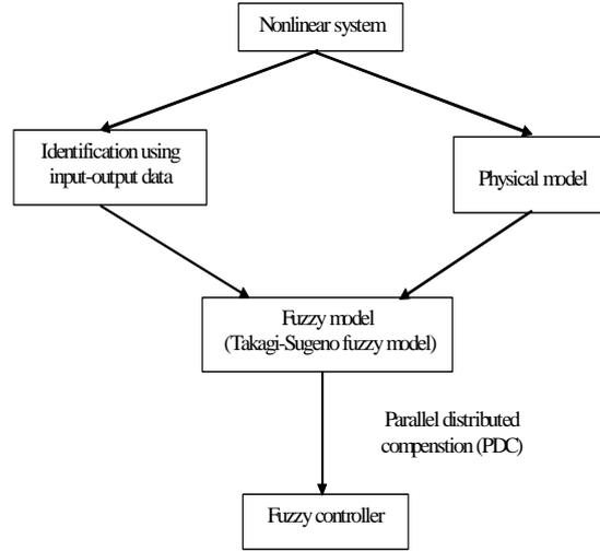
Figure 2.3: Model-based fuzzy control design
