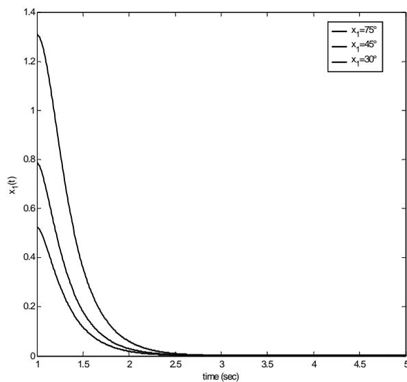
Figure 3.5: Angle response using two-rule fuzzy control and  $M$  changed from 8.0 to 4.0  $kg$ .
