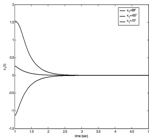
Figure 3.4: Angle response using two-rule fuzzy control and  $m$  changed from 2.0 to 4.0 kg.
