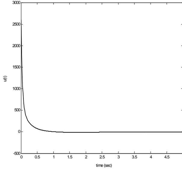
Figure 5.4: Inverted pendulum action evolution without pole placement
