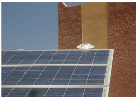
Figure 5. Photo showing the CM11 pyranometer beside the PV generator
