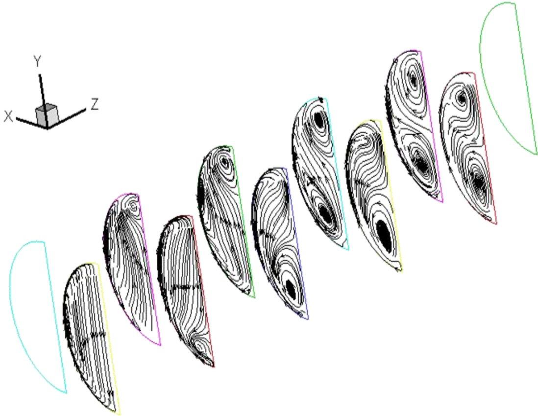
Figure 3.4 : Streamlines at xy-planes of various bends along the S-curved/sinusoidal pipe for  $\dot{m}_m = 9.5 \text{ kgs}^{-1}$  ( $\text{Re} = 12.3 \times 10^4$ ) and  $T_m = 450 \text{ K}$ . The pipe wall was omitted.
