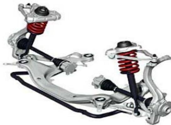
Figure 1. 3 - Suspension de type double triangulation [5]
