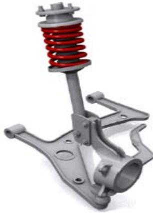
**Figure 1.1** - Suspension de type Mc Pherson [5]
