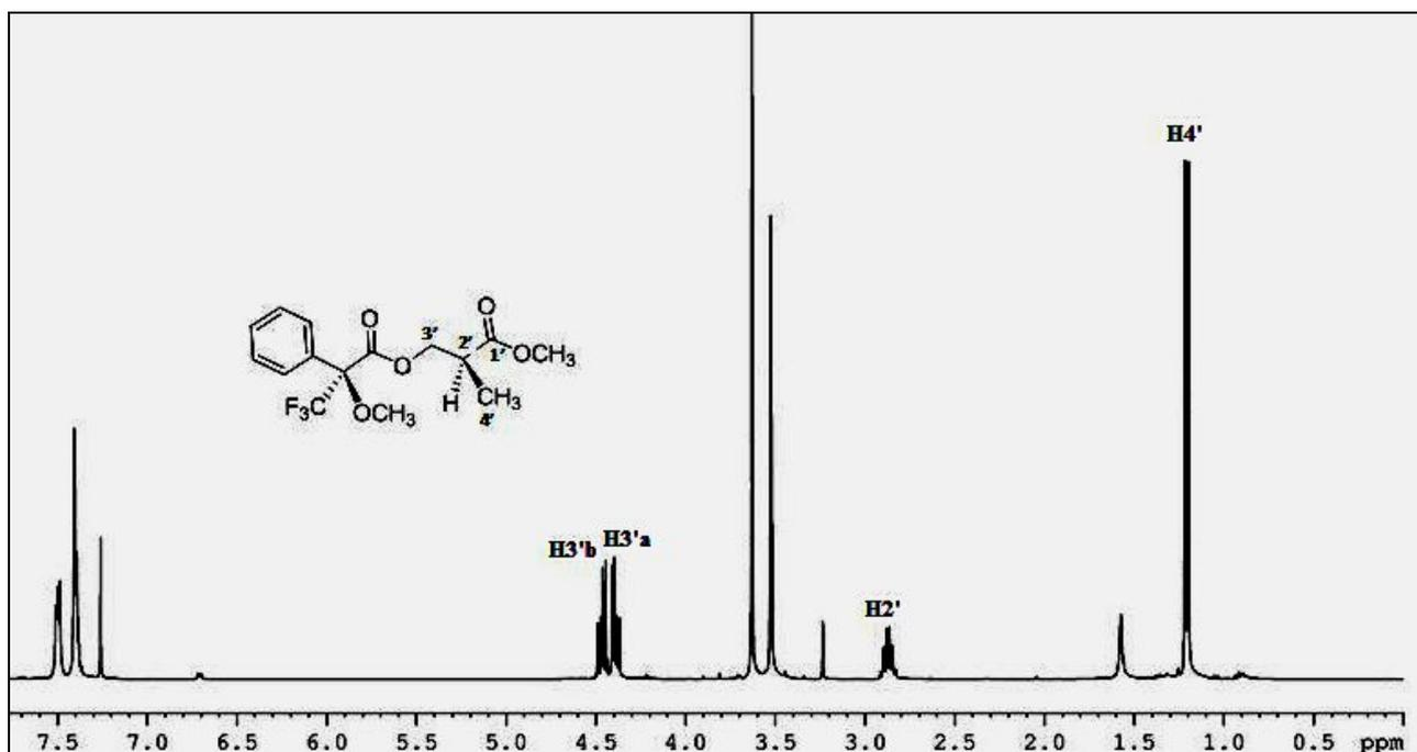
Figure 3.82:  $^1\text{H}$  NMR spectrum of the compound Ia (*S/S*-MTPA ester) in  $\text{CDCl}_3$
