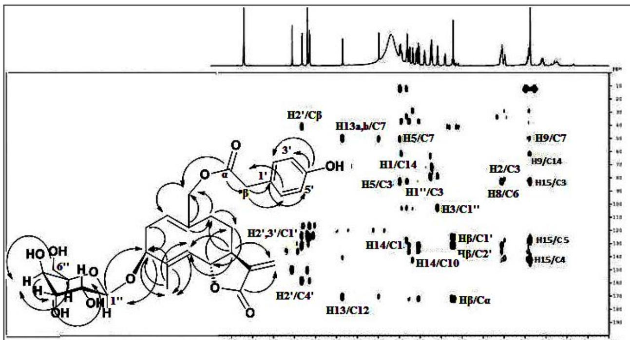
**Figure 3.99:** HMBC spectrum and the significant correlations observed for compound **314** in pyridine- $d_5$
