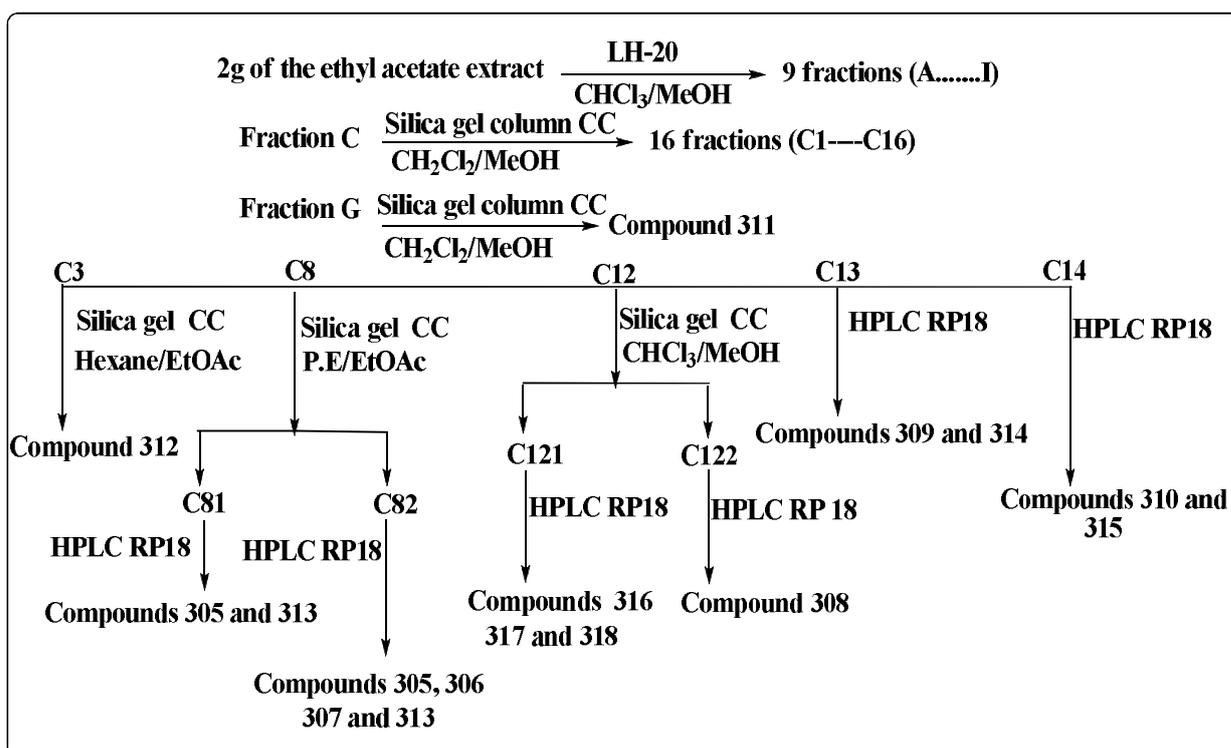
*Figure 3.4: Scheme of the purification of the ethyl acetate extract of the roots*
