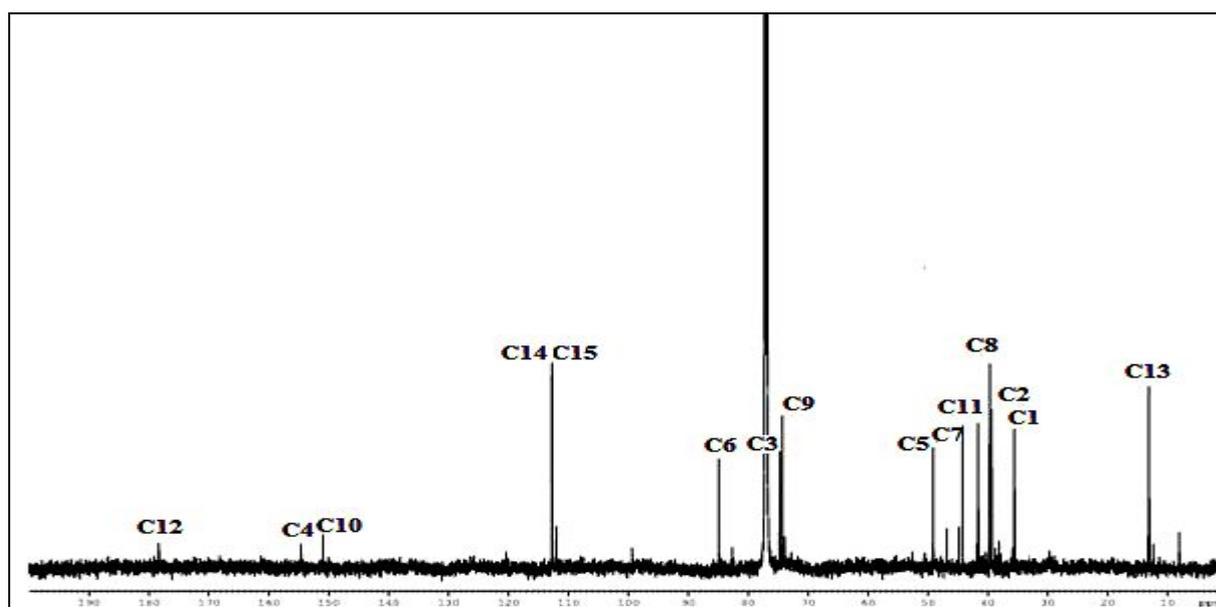
Figure 3.45:  $^{13}\text{C}$  NMR spectrum of compound 305 in  $\text{CDCl}_3$
