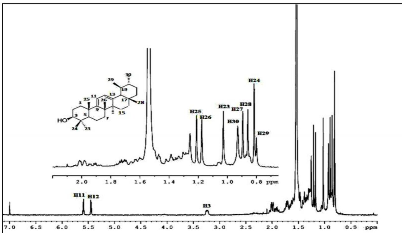
Figure 3.31:  $^1\text{H}$  NMR spectrum of compound 299 in  $\text{CDCl}_3$
