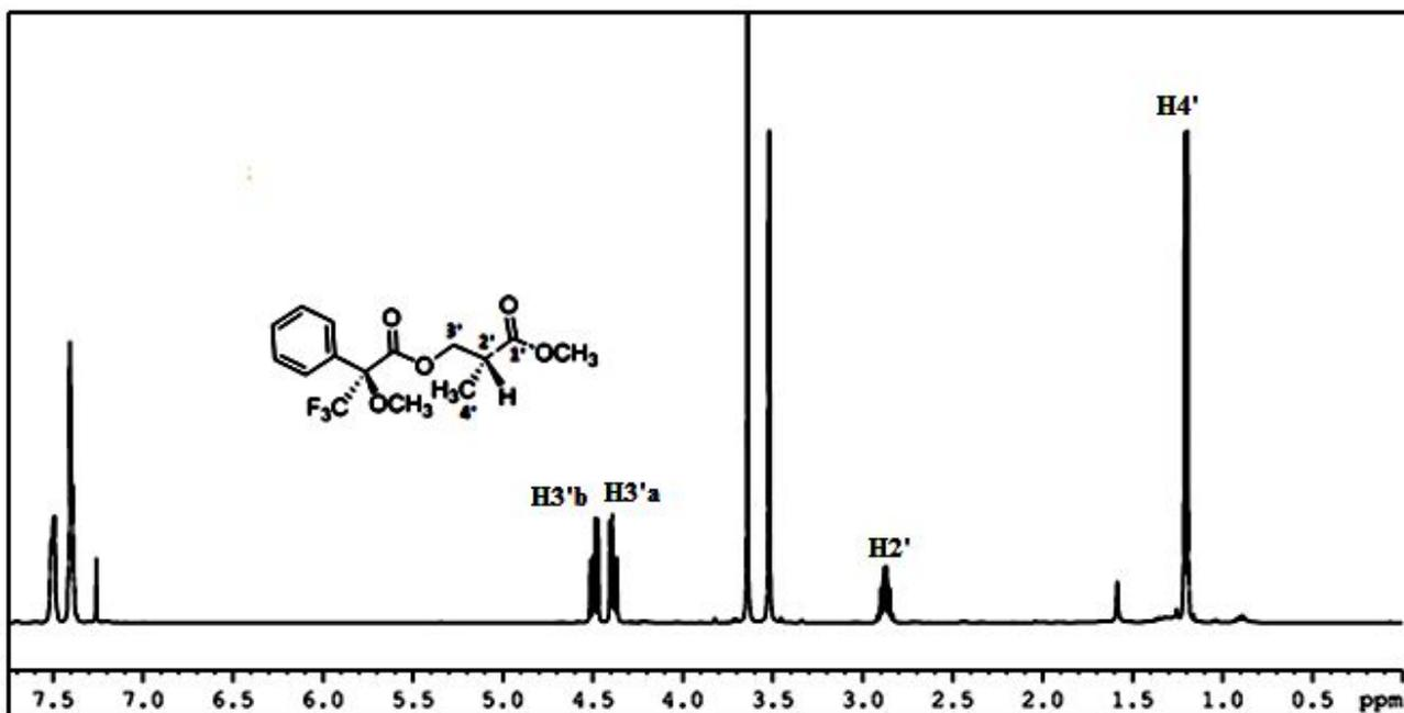
Figure 3.84: <sup>1</sup>H NMR spectrum of compound IIa (R/S-MTPA ester) in CDCl<sub>3</sub>
