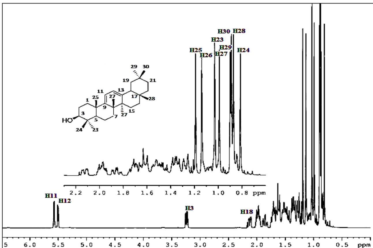
Figure 3.27:  $^1\text{H}$  NMR spectrum of compound 298 in  $\text{CDCl}_3$
