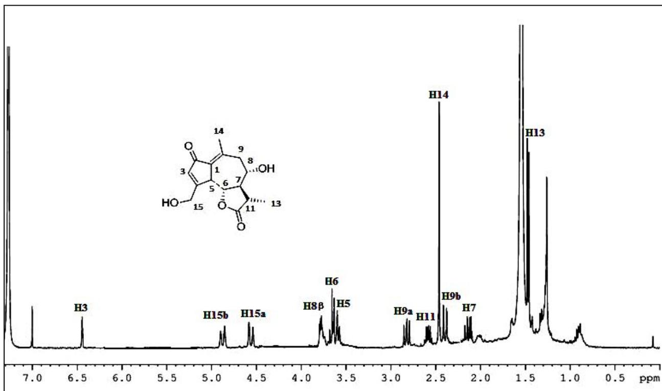
Figure 3.61:  $^1\text{H}$  NMR spectrum of compound 307 in  $\text{CDCl}_3$
