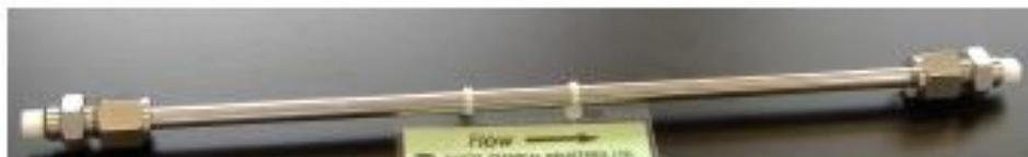
**Figure 1: HPLC column**
